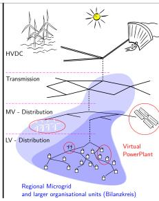
Dynamics driven by inverters and weather, not just synchronous machines and demand. Control distributed, balancing locally.
